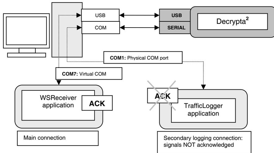
DECRYPTA<sup>2</sup> connected by USB and serial port on different PC
