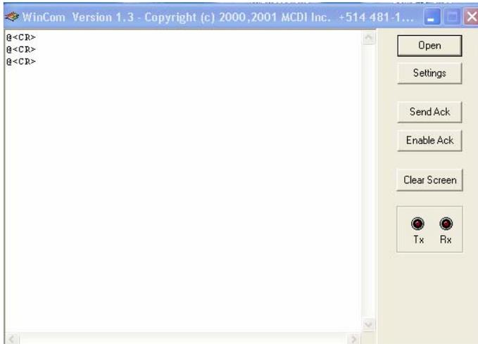
Use WINCOM utility to test communication between computer and DECRYPTA<sup>2</sup>.
